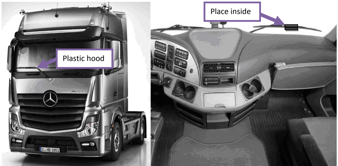
Figure 55. Possible mounting places in trucks
