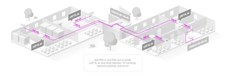
The dual-band, dual-chain 2.4 and 5 GHz wireless radio provides a strong coverage in 360 degrees around it, so you don't have to worry about the placement of the device so much. Putting it on the ceiling eliminates many signal absorption problems, such as the signal being blocked by large TV sets, metal cubicle walls in open space offices, etc.
